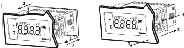
1-Before mounting the device in your panel, make sure that the cut-out is of the right size.
