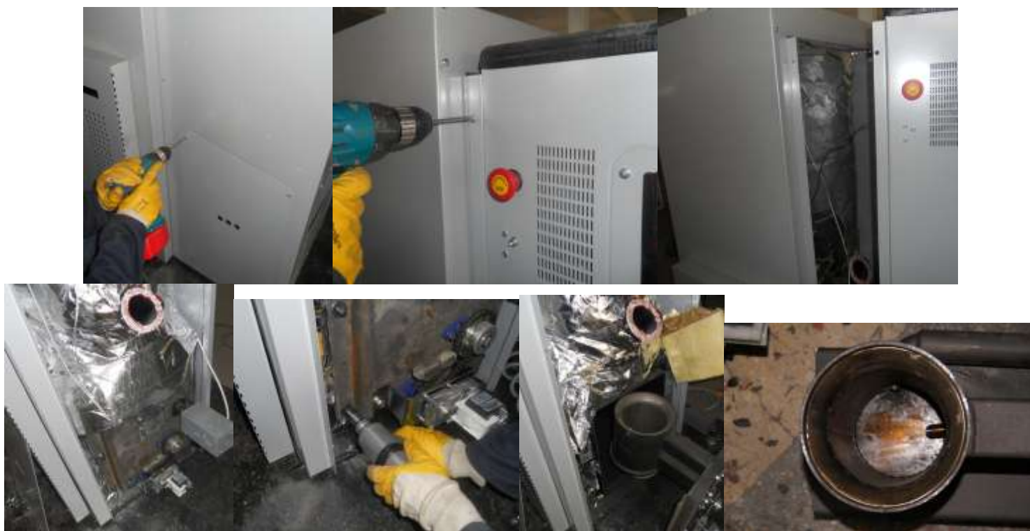
Cleaning of secondary air channels in burnpot and the base of burnpot.
