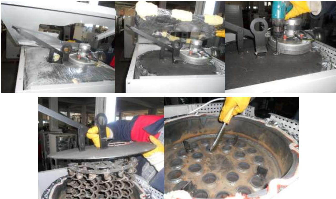
Cleaning of the suction fan and the flue tube
